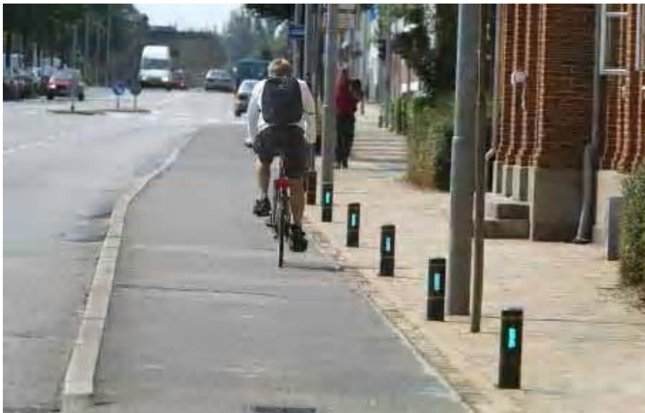
Green wave for cyclists in Odense, with bright green lights flashing on bollards just to the right of the lane to indicate correct cycling speed to achieve all green lights at intersections
